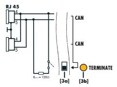
Fig. 3: Termination switch and corresponding indicator LED
