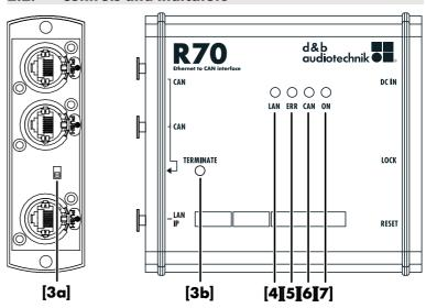
Fig. 2: Controls and indicators
