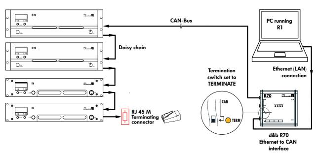
Fig. 5: d&b Remote network (CAN-Bus), wiring example 1 with terminated R70 interface at the "beginning" of the CAN-Bus segment.
