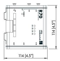
Fig. 8: Wall mounting with dimensions in mm [inch]
