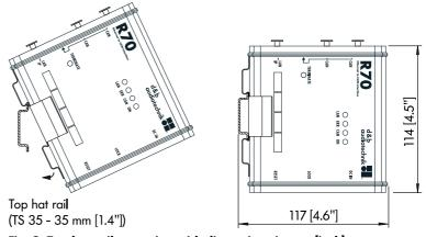
Fig. 9: Top hat rail mounting with dimensions in mm [inch]
