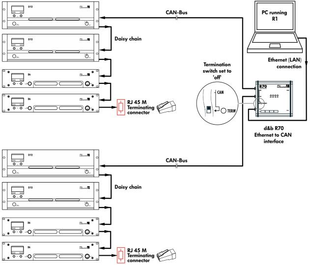
Fig. 6: d&b Remote network (CAN-Bus), wiring example 2 with non-terminated R70 interface within the CAN-Bus segment.
