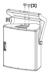
Fig. 5: Attaching the Z5056 M4 Flying bracket to the cabinet
