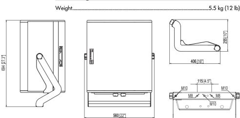
Fig. 2: Z5056 M4 Flying bracket dimensions in mm [inch]
