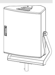
Fig. 7: Z5056 M4 Flying bracket with Z5010 TV spigot
